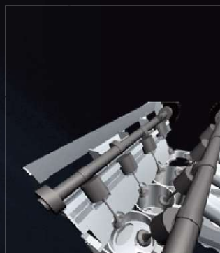
Gas distribution system
